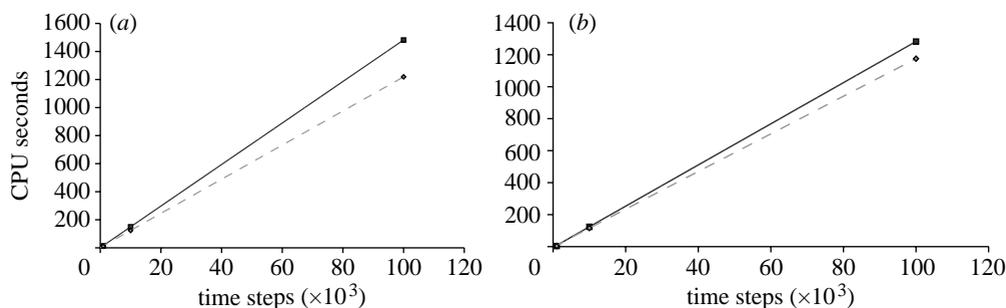
Figure 2. A performance comparison of the time taken (in seconds) by a single machine versus two machines at a time (for BrH) on LONI: (a) 16 (DU; diamonds) versus 8+8 (DU+ZE; squares) processors; and (b) 32 (DU; diamonds) versus 16+16 (DU+ZE; squares) processors.
